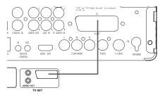
TV Connection (Method 2) – Using S-Video Cable (Not Included) If your TV set has an S-video input jack, you can connect your TV to the S-Video Out Jack ② on the back of the CS receiver. S-video wires don't transport audio signals, so you need an additional audio connection (see note above).
